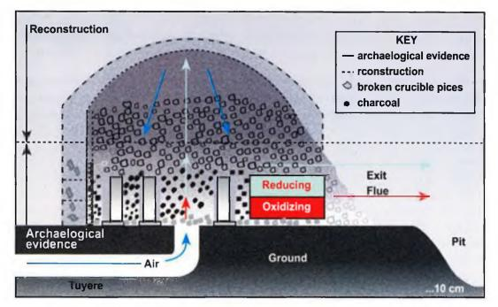
Figure 58: Ironmaking furnace uncovered in Merv (Courtesy: Ann Feurerbach)
