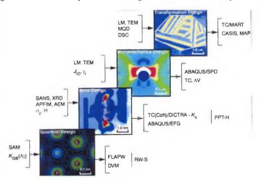
Figure 64: Multiscale modelling is used to link different length and time scales. Both computation and experimental techniques are now available to go from the atomic-through nano-, meso-, micro- to macro-levels (Courtesy: G. B. Olson)
