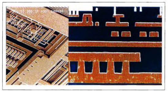
Figure 65: Damascus copper interconnection in a semiconductor device (Courtesy: IBM)
