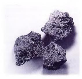
Figure 11: Tama hagana - Special Japanese iron made by the Tatara process (Courtesy: T. Inoue)
