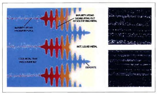
Figure 39: Banding in vanadium containing steels. The dendrites form on solidification and vanadium segregates in the interdendritic space. During subsequent cooling and heating cycles this forms the basis for carbide formation and the ultimate pattern (Courtesy: J. D. Verhoeven)
