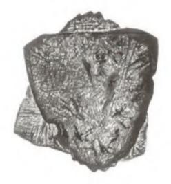
Figure 30 : **Sket**ch of etched structure of wootz ingot revealing dendrites
