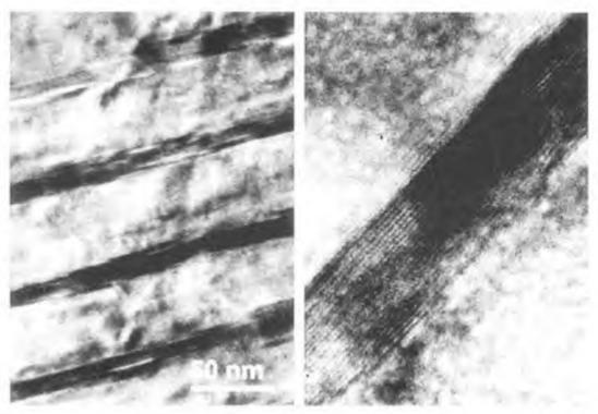
Figure 62: Detection of nanowires in Damascus steel. High resolution transmission electron microscopic images reveal nanowires of cementite several hundred nanometers in length (Courtesy: Werner Kochmann)
