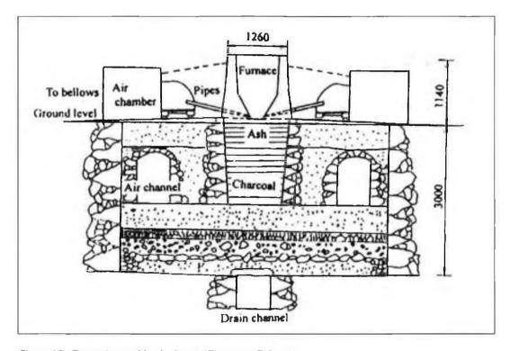
Figure 10: Tatara ironmaking in Japan (Courtesy: T. Inoue)
