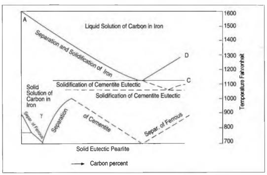
Figure 12: Iron-carbon (Fe-C) diagram (first phase diagram of any alloy to be established, done by Roberts-Austen in 1898 after whom austenite came to be named)
