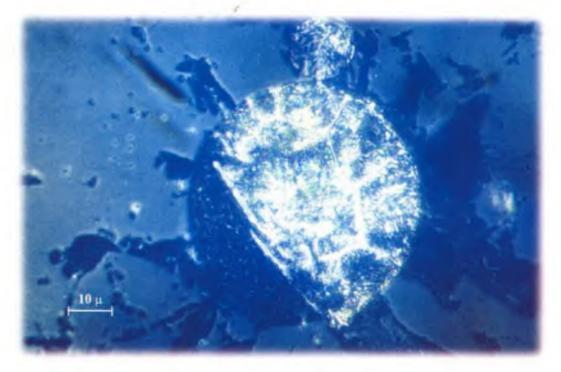
Figure 54: Microstructure of a cross section of crucible from Mel-siruvalur showing globule of steel
