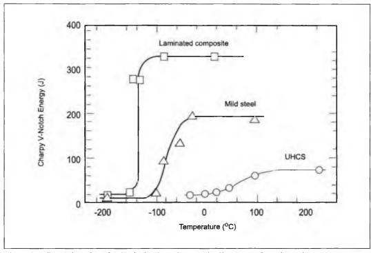
Figure 49: Illustration of toughening by laminated composite (Courtesy: J. Wadsworth)
