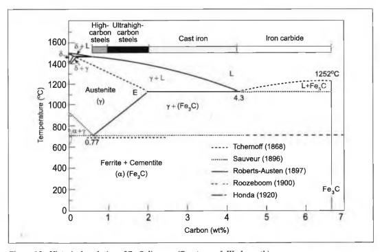
Figure 13: Historical evolution of Fe-C diagram (Courtesy: J. Wadsworth)
