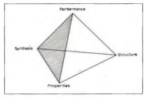
Figure 60: Materials tetrahedron indicating relation among structure, properties, processing and performance
