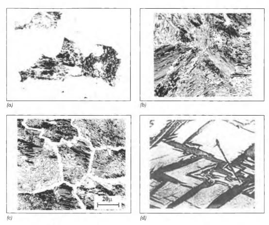
Figure 14: Microstructures of steels (a) ferrite grains in a hypoeutectoid steel, (b) pearlite lamellae in an eutectoid steel (c) pearlite with cementite at grain boundaries in a hypoeutectoid steel (d) martensite in quenched steel (Courtesy: L. E. Samuels)
