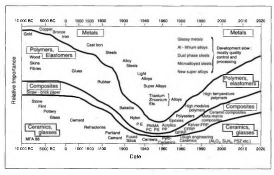
Figure 4: The intensity of the use of materials over ten millennia (after M. F. Ashby)
