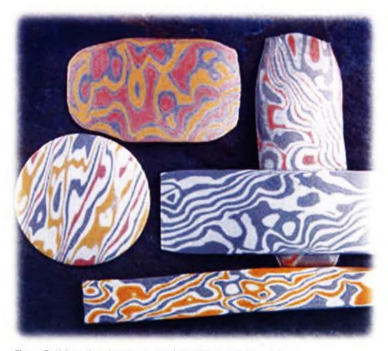
Figure 47: Mokume Gane from Japan - wood like patterns created in metals
