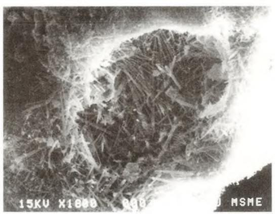
Figure 56: Scanning electron micrograph of mullite network in the refractory of the crucible (Courtesy: Thelma Lowe and Gareth Thomas)
