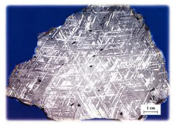
Figure 7: Widmanstatten pattern in meteoritic iron. Note the beautiful geometry of the pattern and the scale visible to the naked eye
