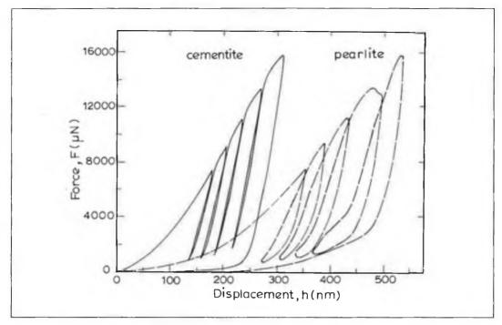
Figure 63: Nanoindentation of cementite and peralite. Force-displacement curves indicate a pronounced hysteresis in pearlite and none in cementite (Courtesy: Werner Kochmann)
