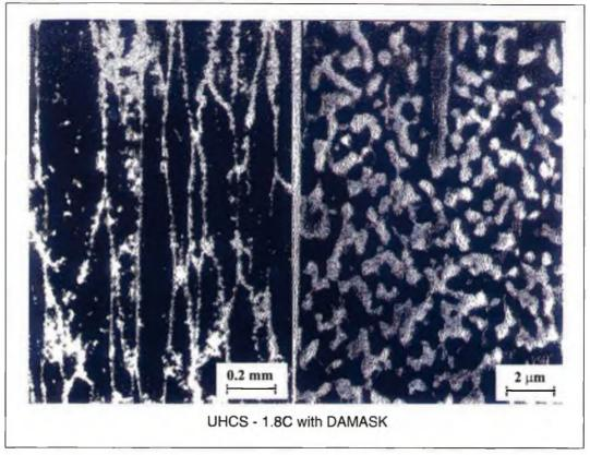
Figure 38: Fine grained microstructure of ultra-high steel (Courtesy: O. D. Sherby and J. D. Wadsworth)
