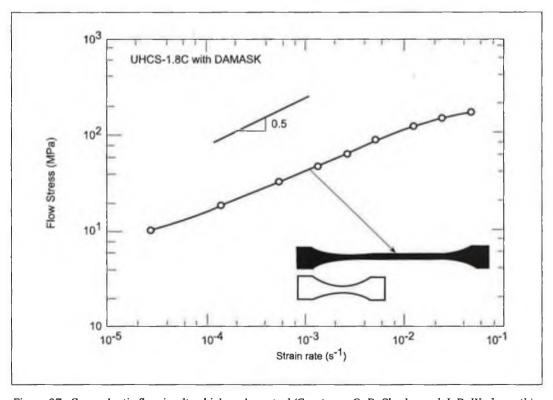
Figure 37 : Superplastic flow in ultra-high carbon steel (Courtesy : O. D. Sherby and J. D. Wadsworth)
